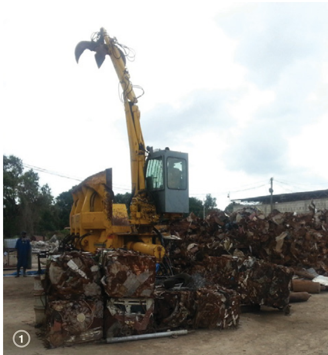
1. Excavation grapple used to load material onto a container.
